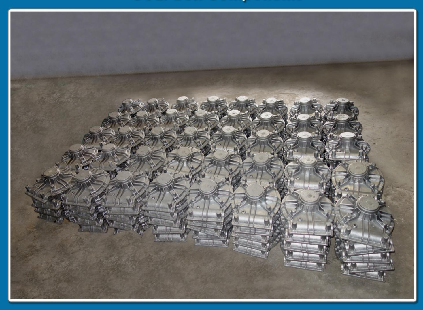
Gravity Die Casting Pneumatic Cylinder Machined Components
